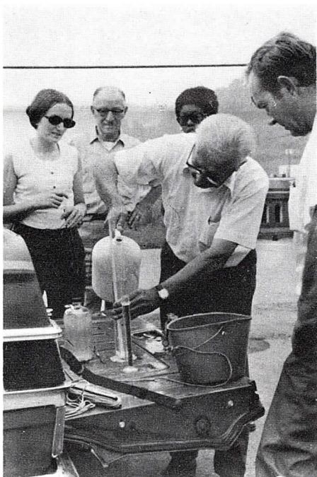
Mike Watts makes field test for oxygen content of samples using his portable testing equipment.
