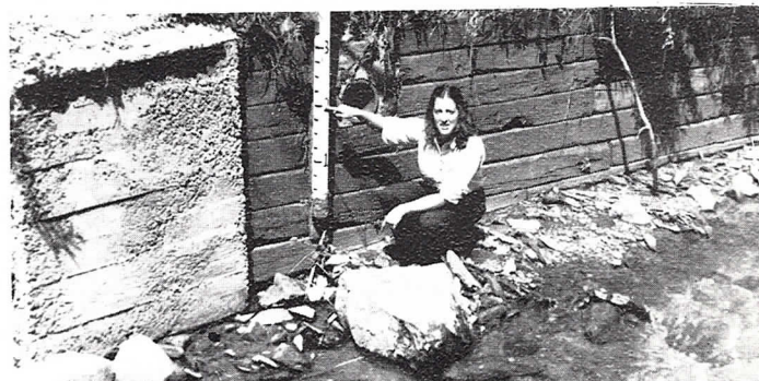
TCWA's Susann Seibel identifies one of the 9 stream gauges (and two precipitation stations) which TCWA operates to obtain base data for the area's stormwater plan.
