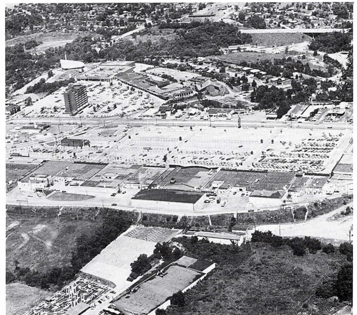
Without stormwater controls, large sections of impervious surfaces such as shown here can cause runoff that can rip apart stream channels, depositing sediments below in Turtle Creek's flood control channel.
